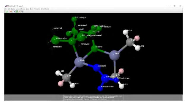
A last step is to prepare templates with ring flipped for optimal TS structure development. To do so, select an atom of the ring to flip and the four atoms directly connected and select "flip the ring". With these instructions, both flipped templates will be produced.
