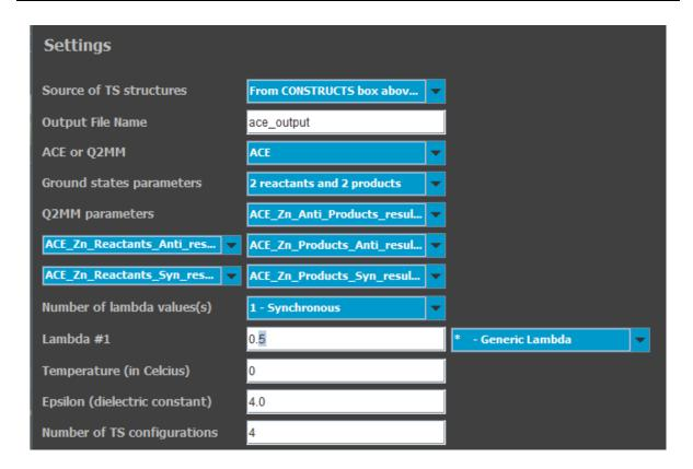
You can now run the workflow again which will generate all the necessary files ready to be used by ACE.
