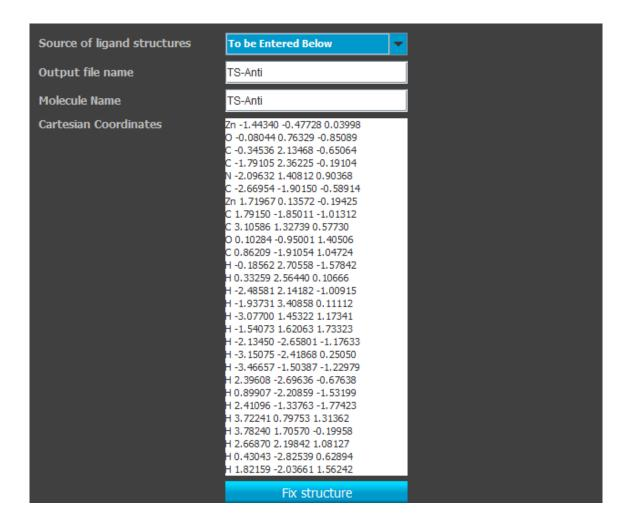
To visualize the structure, click on "Fix structure". In this current case, we are converting the  $NH_2$  of the catalyst reported into  $N(Me)_2$  which we believe would be more representative of the catalysts under investigation. To do so, two hydrogens (16 and 17) are converted into methyl. To identify the atom number, you may click on "Preview". Before the instruction to add two methyl groups, the structure looks like this:
